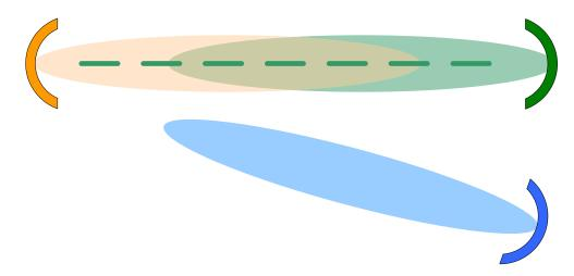
The blue antenna is out of alignment and will not receive or transmit effectively with the orange node. An additional antenna and radio could be used at the orange location, turning this into two separate point-to-point links.
