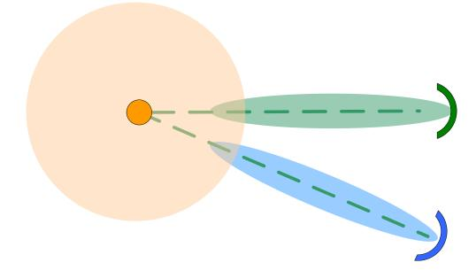
Since the path budget includes the sum of the gains of the antennas at both ends of any given path, the full benefit of the high gain at one end will still be applicable. This hybrid arrangement allows multiple remote nodes to be located anywhere within range as long as they point in the direction of the master node. This alignment is much less difficult since the master side requires only vertical adjustment.
