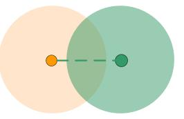
Small vertical (*omni-directional*) antennas typically have gains of between 5 dBi and 9 dBi but exhibit **no directivity in the horizontal plane**. Thus, most of the power of the transmitter is wasted and never reaches the receiver. There must however be some difference between the 5 dBi and 9 dBi models and, it is a function of their **vertical** directivity.
