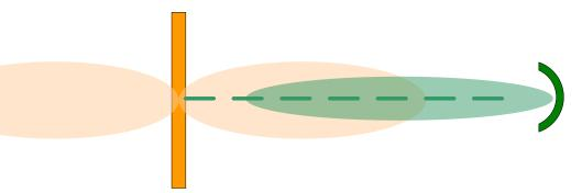
The gain of the special omni might be as much as 15 dBi providing a 2X range improvement over a more standard 9 dBi. The disadvantage is that the narrow vertical radiation pattern of the high gain omni means that vertical alignment is quite critical.
